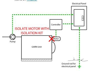
Dielectrically isolate any pumps directly connected to the GARN unit:
