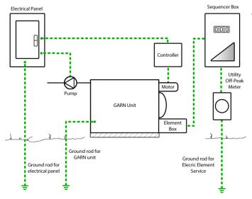
The goal is to build to a single-ground point through the element box, the sequencer box, and ultimately the ground rod associated with the electric heating element service. To do this:
