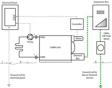
Ensure that the unit is grounded through the element box by attaching the ground wire to one of the studs in the electric element box. The ground wire must ultimately run back to ground of the meter/panel supplying power to the electric elements.
