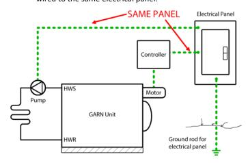
If a pump connected directly to the GARN unit is wired to a different panel, then the pump **OR** blower motor **or both** must be electrically isolated:
