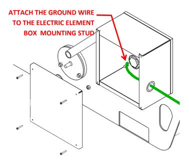
Single-point grounding with electric heating elements is now complete.
