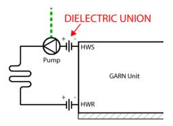
By installing dieletric unions (or equivalent) on or near the Hot Water Supply (HWS) and Hot Water Return (HWR) connections of the GARN unit, electric isolation is achieved for any and all components connected downstream.
