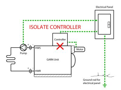
A simple solution to isolate the controller is to remove the controller from its steel stud mounting, screw a piece of plywood into the steel studs, then mount the controller to the plywood Make sure the new controller mounting screws are not in contact with the steel studs. Plywood is an effective electric isolator.
