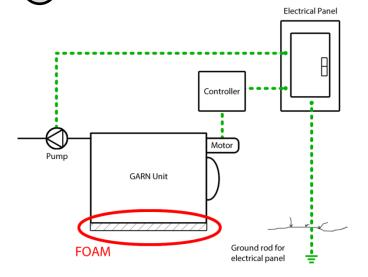
Isolate the blower motor with a blower motor isolation kit: (Part #: P-0125 on www.garnparts.com). Installation instructions for the isolation kit can be found on PAGE 8.
