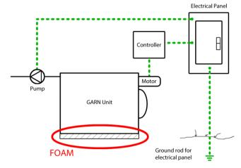
Check to ensure that the blower motor and ANY pump that IS NOT dielectrically isolated from the GARN unit is wired to the same electrical panel:
