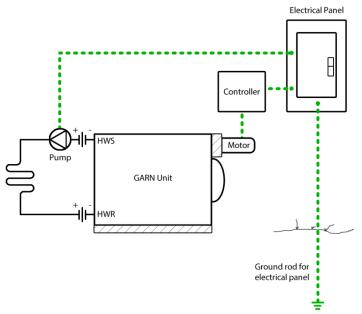
The GARN unit is now fully electrically isolated. Anode rods are not needed. If the installation changes over time and other electrical devices are installed on or near the GARN unit that are wired to ground, keep these concepts in mind and isolate appropriately.
