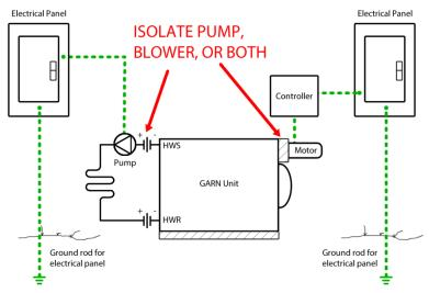
Isolate the blower motor with a blower motor isolation kit: (Part #: P-0125 on www.garnparts.com). Installation instructions for the isolation kit can be found on PAGE 8.
